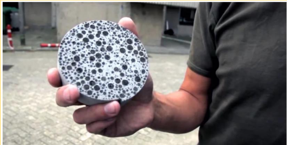
Piece of the Bio Concrete (self-healing concrete)
